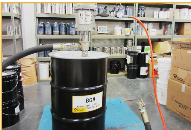
Pump mounted down on scale.
