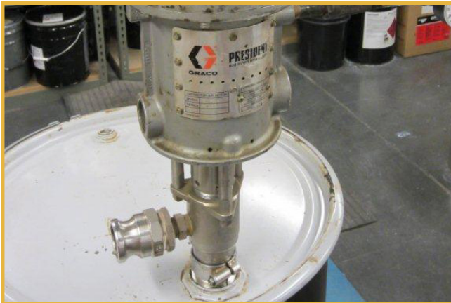
The pump is inserted into the 2" bung opening in the lid of the drum.
