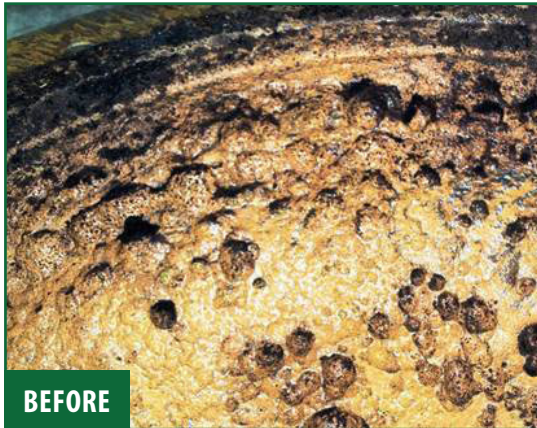
Heat exchanger floating head before and after pits in steel were filled using Novocoat EP3900 Machinable Paste . Novocoat SC5400 Lining applied as topcoat.
